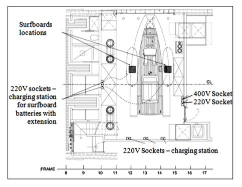
Figure 3: Plan of the garage showing the power outlets
