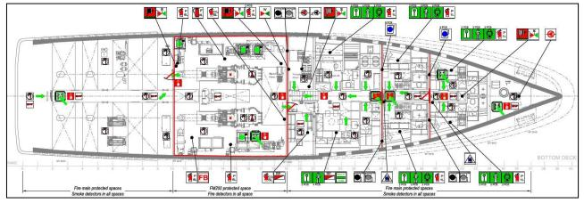
Figure 7: Extract of Fire and Safety Plan – Bottom Deck
