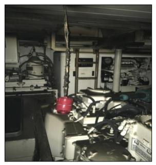
Figure 8: Heat Detector located above the starboard side engine
