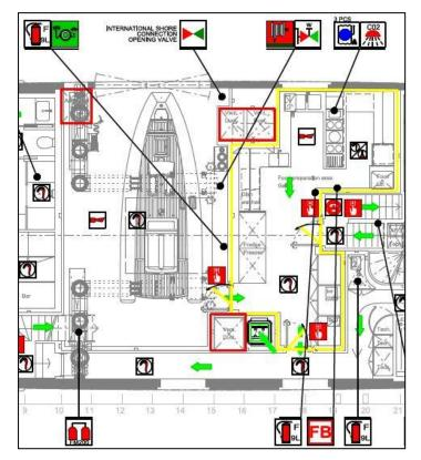
Figure 4: Extract of fire and safety plan depicting the garage and galley
