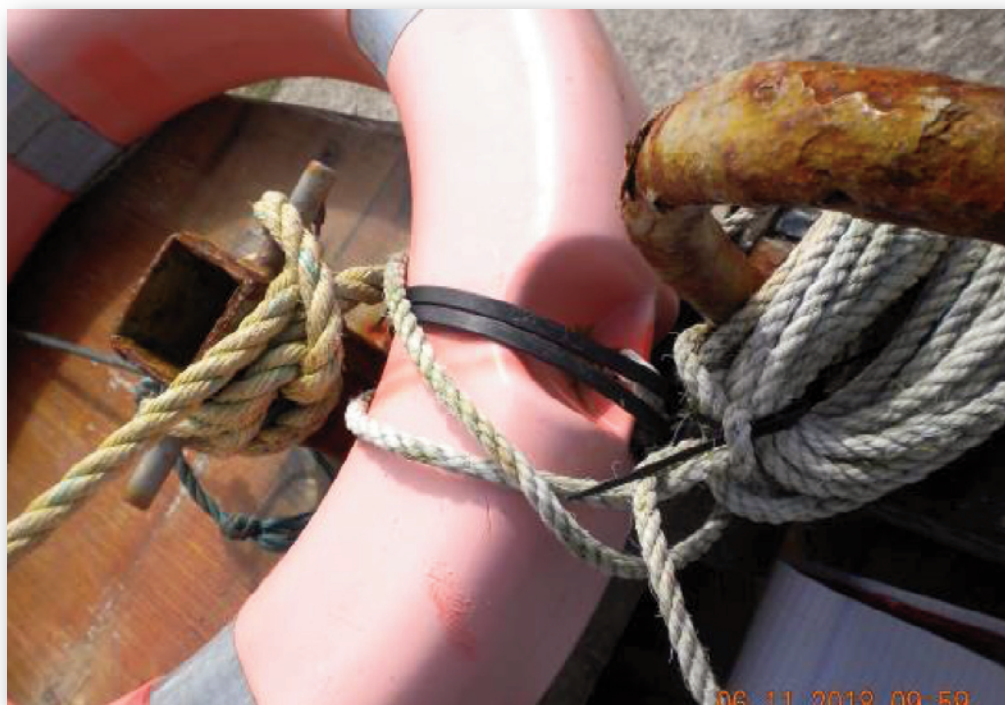
Photograph No. 8: Cable tie used to secure lifebuoy to vessel.
