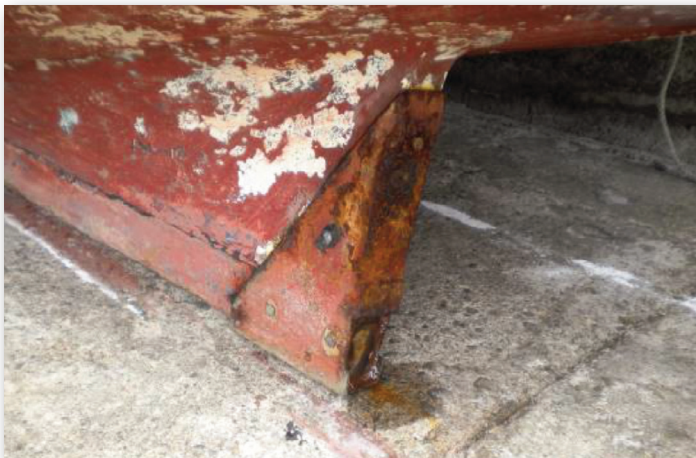
Photograph No. 6: Steel shoe covering stern tube opening.
