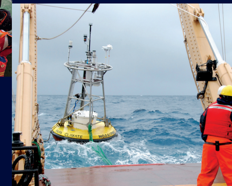
Surface element of a long term deep sea mooring, equipped with pH and other CO 2 relevant sensors, deployed in the North Pacific Ocean. Dr M. Cronin, PMEL NOAA.
