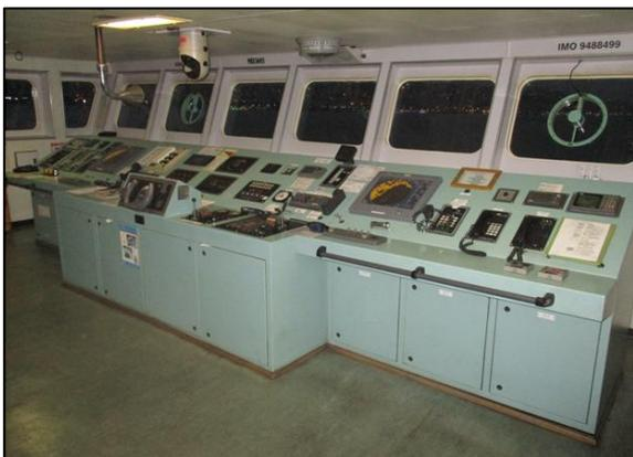
**Figure 1: Layout of the main console and navigational equipment**
