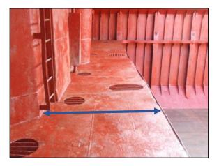
Figure 5: A much wider forward tweendeck platform inside cargo hold no. 2 (although the absence of physical and symbolic barrier systems are apparent)
