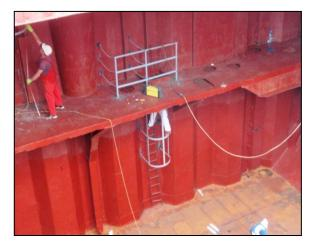
Figure 5: Physical barrier systems fitted after the accident
