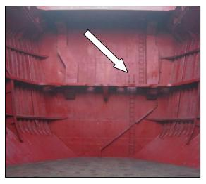
Figure 2: Forward bulkhead and access ladders
