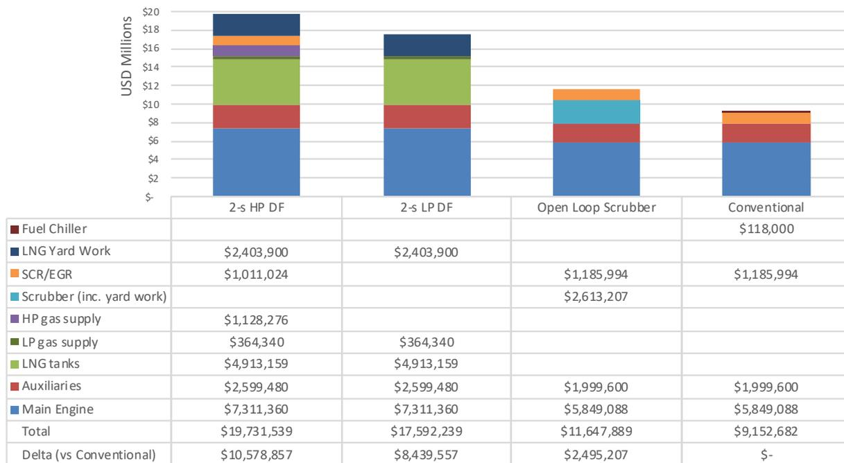
The additional CAPEX for each 8,000 CEU vessel configuration option over the conventional vessel is:
