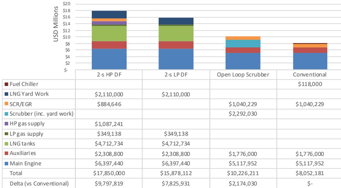
The additional CAPEX for each 6,500 CEU vessel configuration option over the conventional vessel is:
