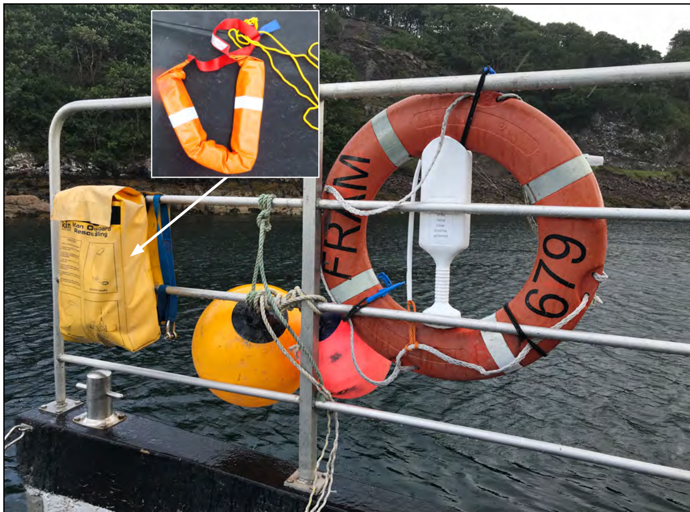
Figure 5: Person overboard rescue sling and lifebuoy with 18m rope line
