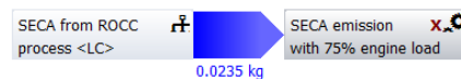
Figure 5.7 1 kg of SECA fuel modelled by processing from heavy fuel oil or residue oil by a residue hydrocracker using heat and electricity in a catalytic reactor.
