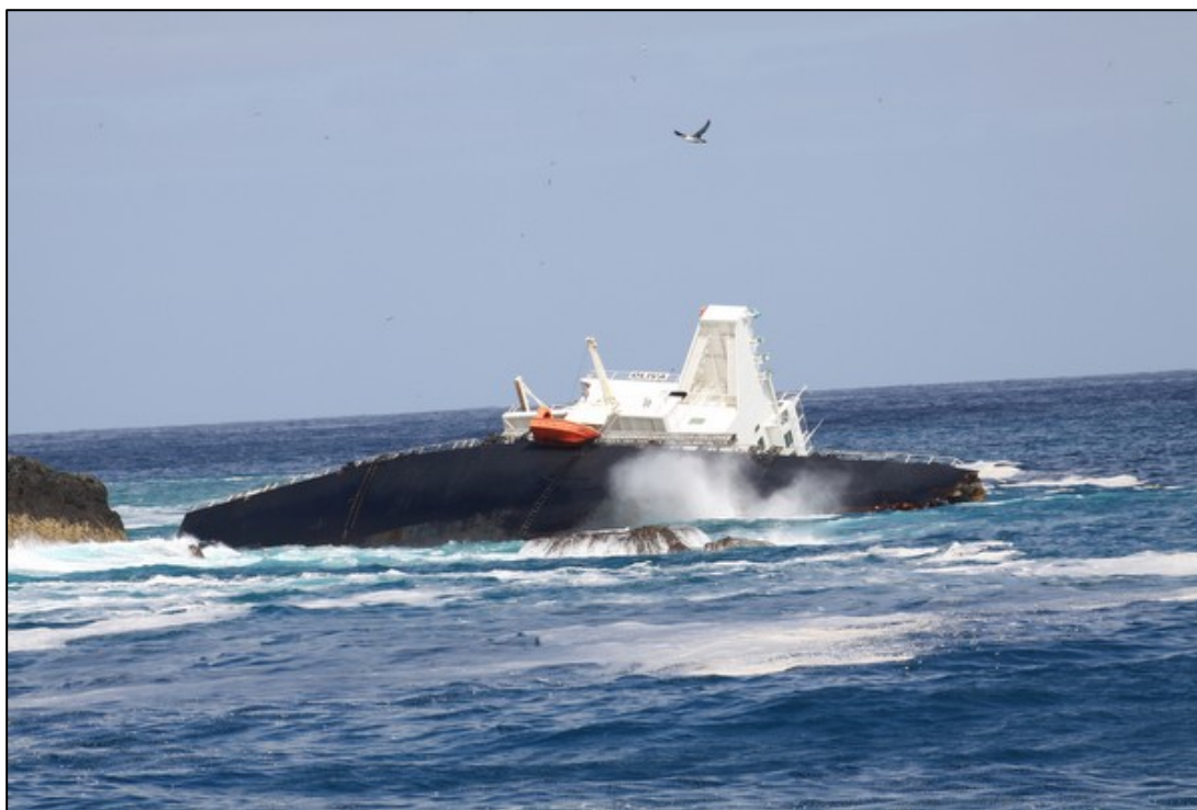
Figure 9: Oliva 's aft section following the hull failure
