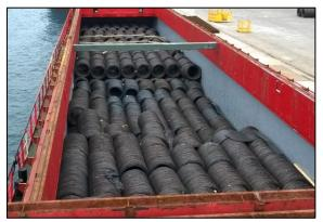
Figure 1: Steel coils stowed in the cargo hold
