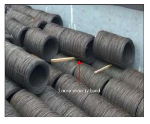
Figure 4: Photo showing a loose security band
