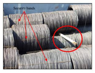
Figure 2: Security bands and 4" x 4" timber used to wedge the steel coils
