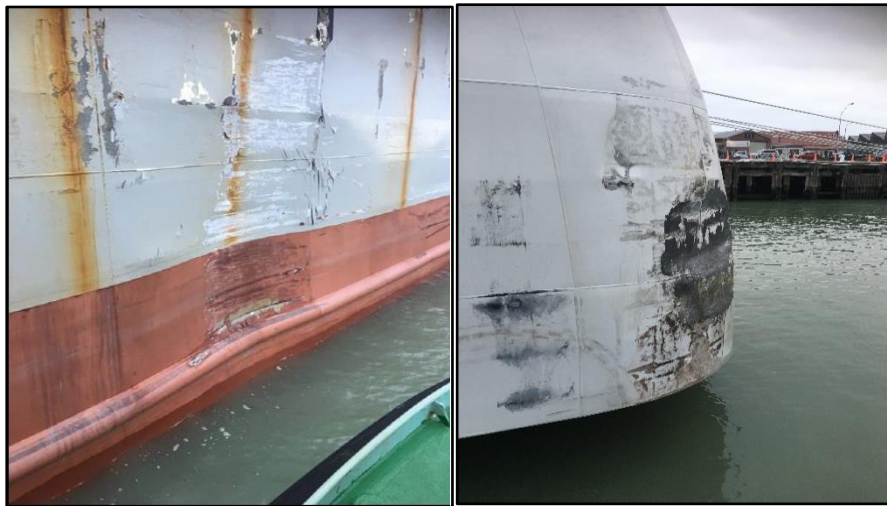
Figure 4 Damage sustained by the Milburn Carrier II (left) and the Seabourn Encore (right)
