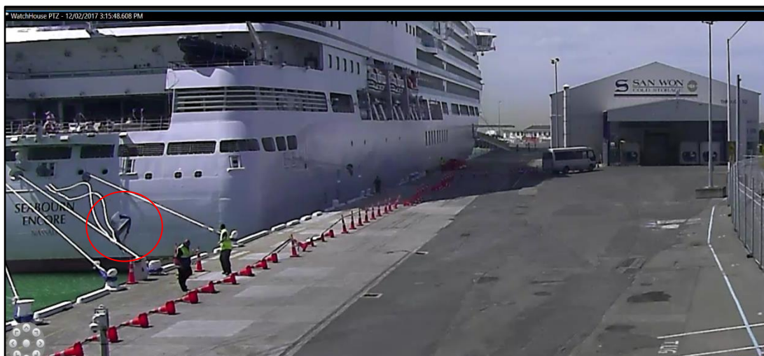
Figure 2 Failure of bollard 26 with two mooring lines attached
