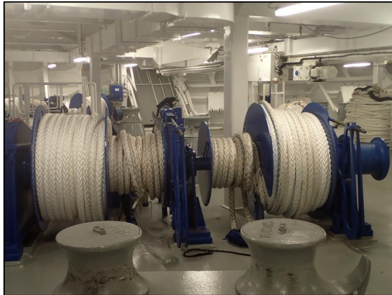
Figure 6 Split drum mooring winch used to secure mooring lines on board the Seabourn Encore
