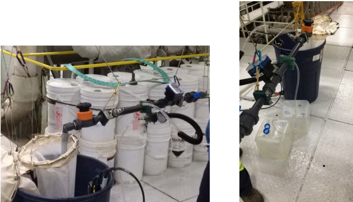
Figure 4. Photographs of sample filtration system using plankton nets.
