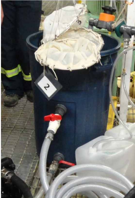
Figure 5. Sample bin with bulk head connectors for out flow of sample ballast water into the bilge.
