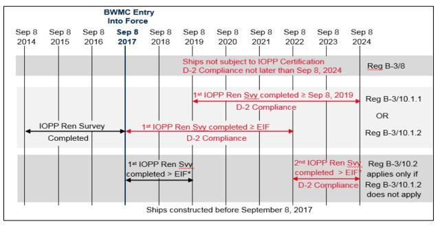
The amendments to regulation B-3 of the BWM Convention, which enters into force on October 13, 2019, requires ships constructed on or after 8<sup>th</sup> September 2017 to comply with the D-2 biological standard upon delivery. Referring to above diagram, ships constructed before 8<sup>th</sup> September 2017 are to comply with the D-2 standard at their **first** MARPOL IOPP Renewal Survey completed on or after:
