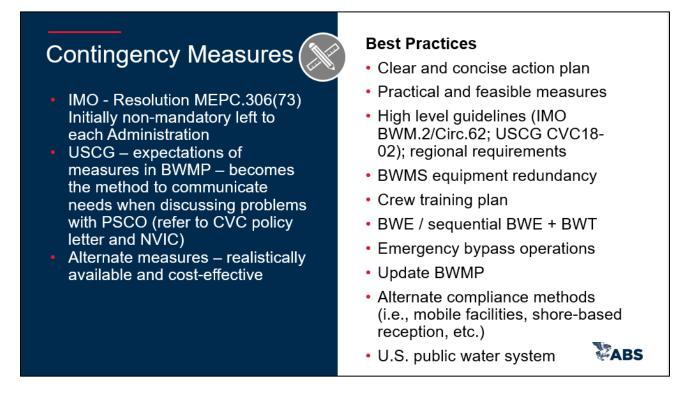
Well planned BWM contingency measures allow shipowners, operators and crew to identify, practice and implement the BWM strategy and be prepared for unexpected circumstances (i.e., inoperable BWMS, equipment failures, etc.). This could avoid unnecessary downtime for the vessel (i.e., delay at berths or ports, inability to continue cargo operations, etc.) and help avoid economic and/or commercial impacts.
