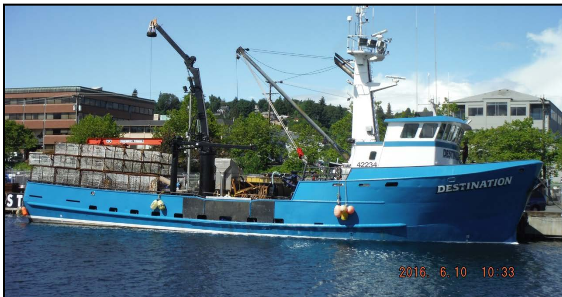
Figure (6): Starboard Profile Showing 9 Freeing Ports
