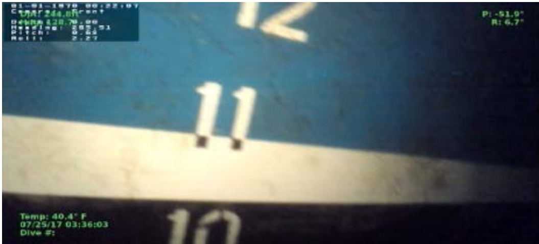
Figure 72. ROV imagery showing the DESTINATION's draft marks. Photo provided by Coast Guard Dive Locker West.
