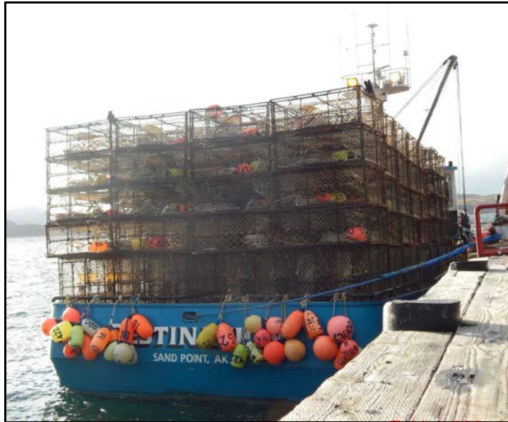
Figure 56. DESTINATION's typical pot loading condition. Undated photo taken and provided by former crewmember.
