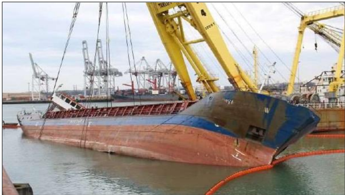
Figure 15: The vessel being lifted upright by a heavy lift at the shipyard
