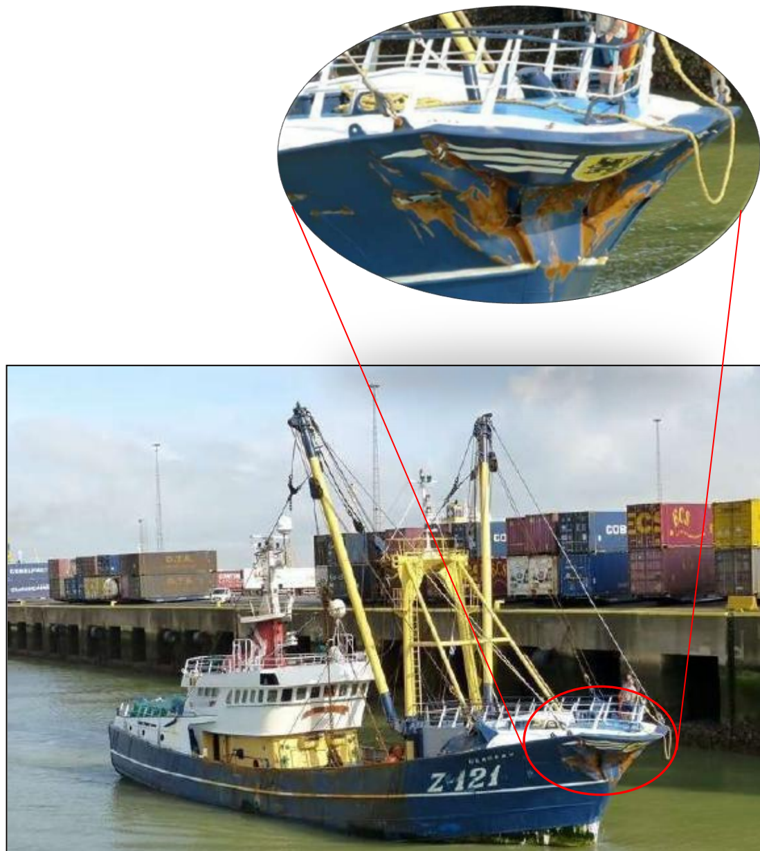
Figure 12: Damages to the fishing vessel's bow area
