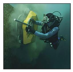
Figure 3.1: Underwater hull cleaning with no capture system evident Source: AUSMEPA (2010).
