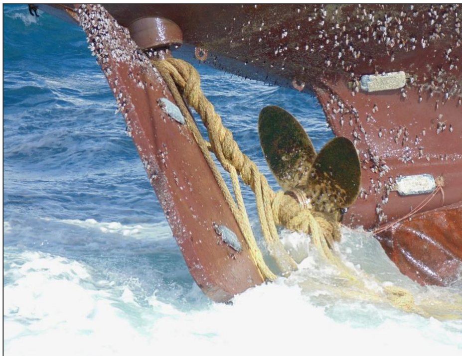
Figure 15: Mooring rope fouling one of the propeller blades and the rudder stock
