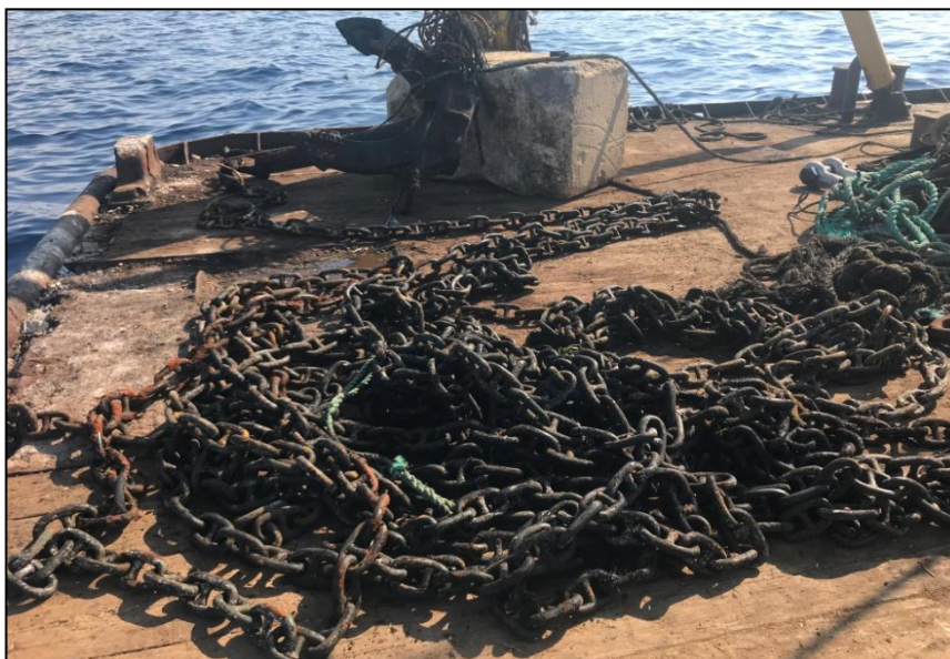
Figure 13: Anchor cable and starboard anchor after being retrieved by the salvor
