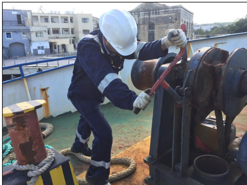
Figure 16: Jammed port side windlass brake
