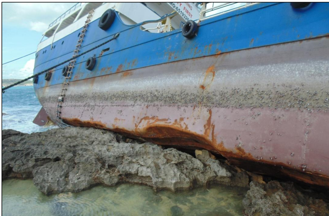
Figure 8: Bottom shell plating set in following the grounding
