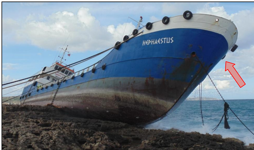
Figure 6: Hephaestus ground with her port anchor and chain missing
