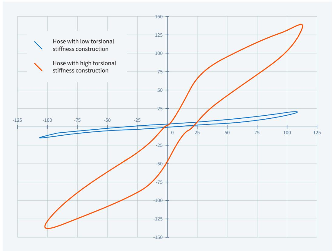
**Table 3.1:** Qualitative comparison of torsional stiffness for different hose constructions
