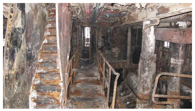
Fire damage of engine room's upper level (looking forward).
