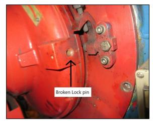
Figure 3: Broken locking pin
