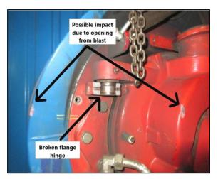
Figure 2: Cracks to the mounting and damaged upper hinge
