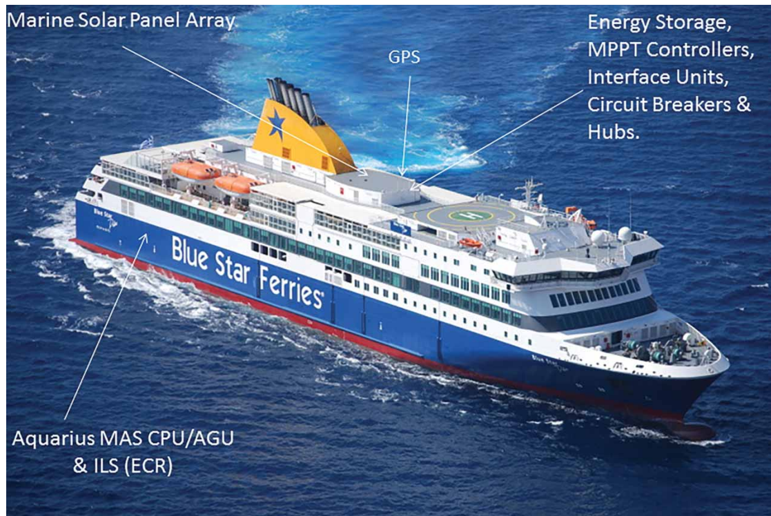
Figure 2. Marine solar power system equipment locations on Blue Star Delos. The picture of the ship is used with the permission of Blue Star Ferries.
