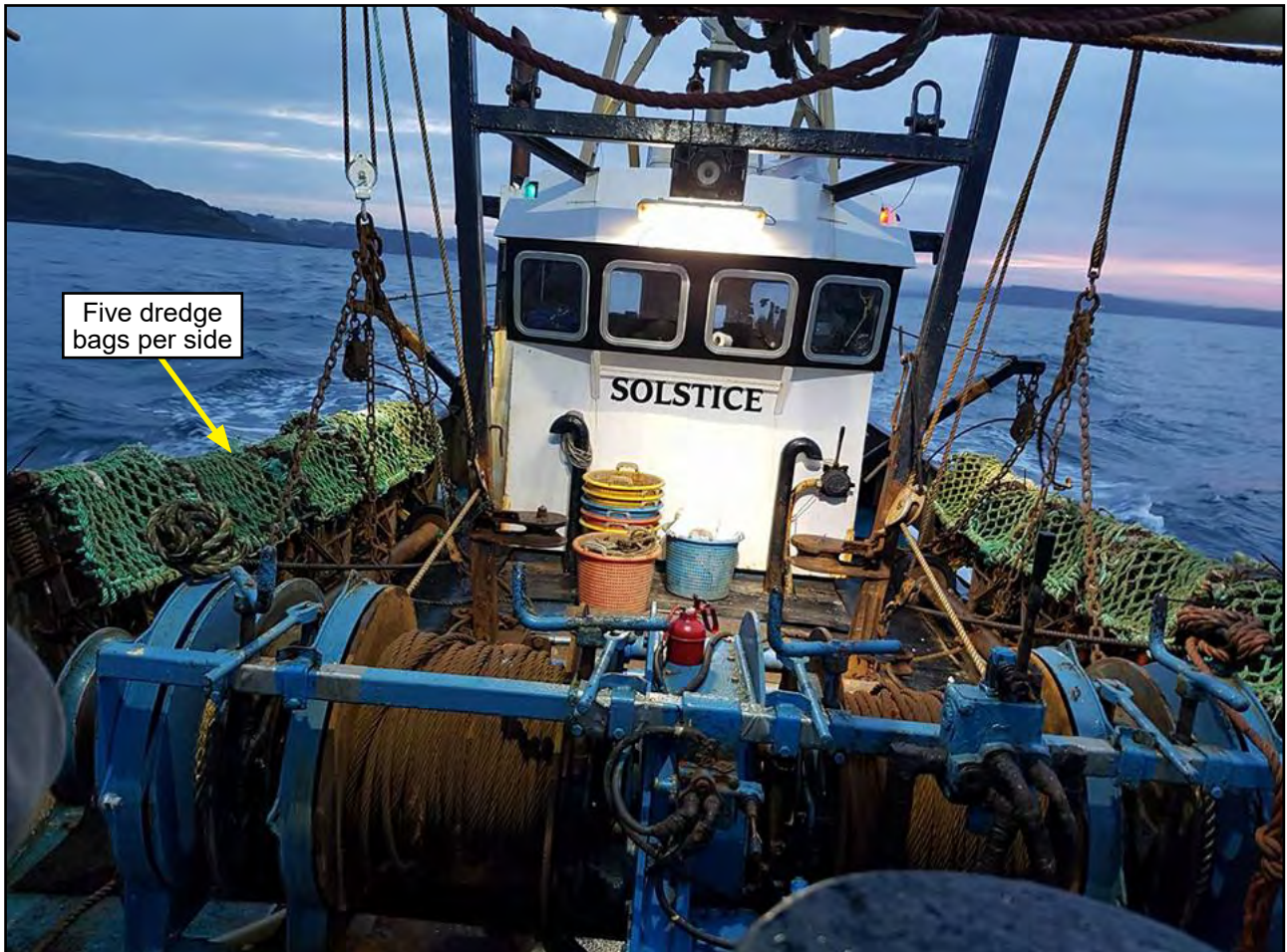
Figure 16: Modifications carried out to Solstice in 2017 to improve dredging method
