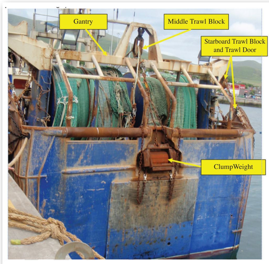
Photograph No. 2: Stern of vessel. Annotated to indicate the Gantry, Middle Trawl Block, Clump Weight and the Starboard Trawl Block and Trawl Door.
