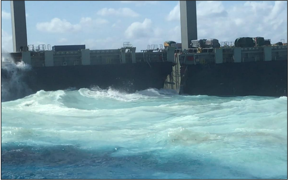
Figure 6: Kea Trader 's structural failure, in way of frame 92
