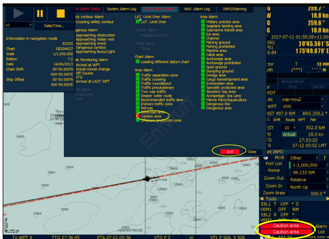
Figure 10: Reconstruction of ECDIS image showing caution area alarm
