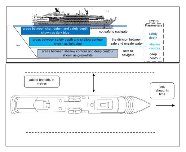
Figure 6 Diagram showing ECDIS safety parameters
