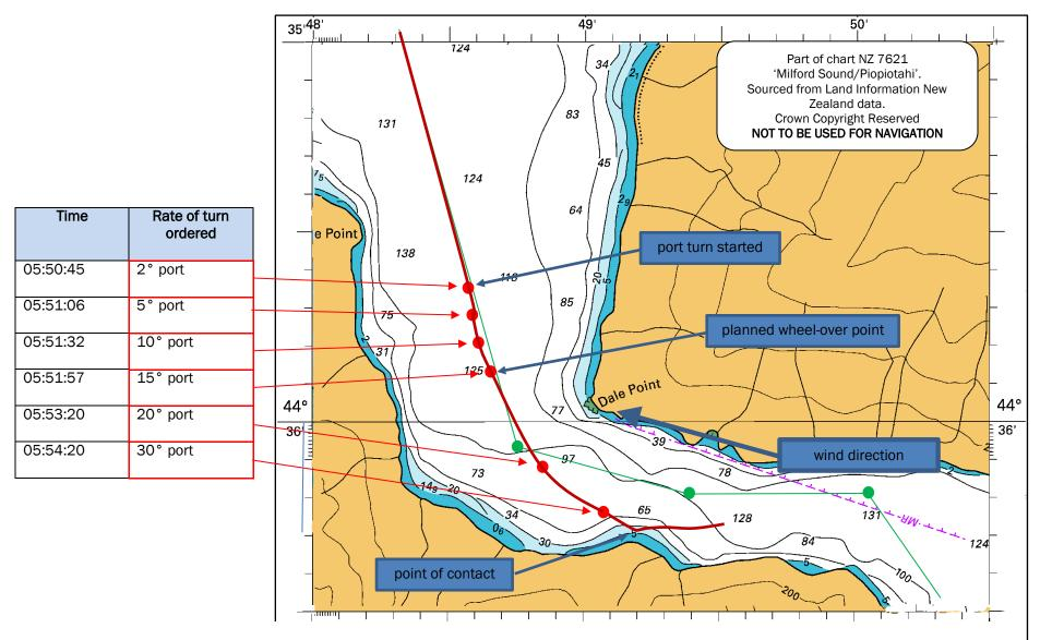
Figure 3 The *L'Austral*'s course around Dale Point with rates of turn as ordered
