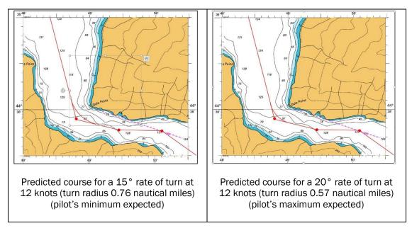
Figure 5 Chartlets showing typical tracks for rounding Dale Point
