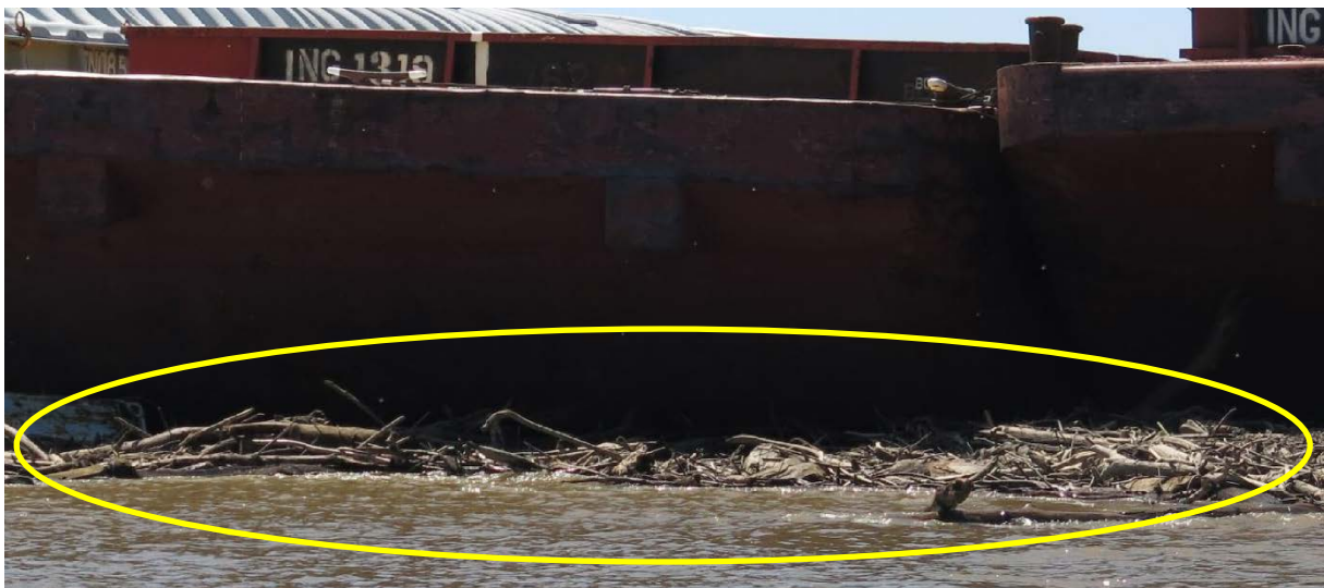
Accumulating debris (circled) under the rakes of fleeted barges.
