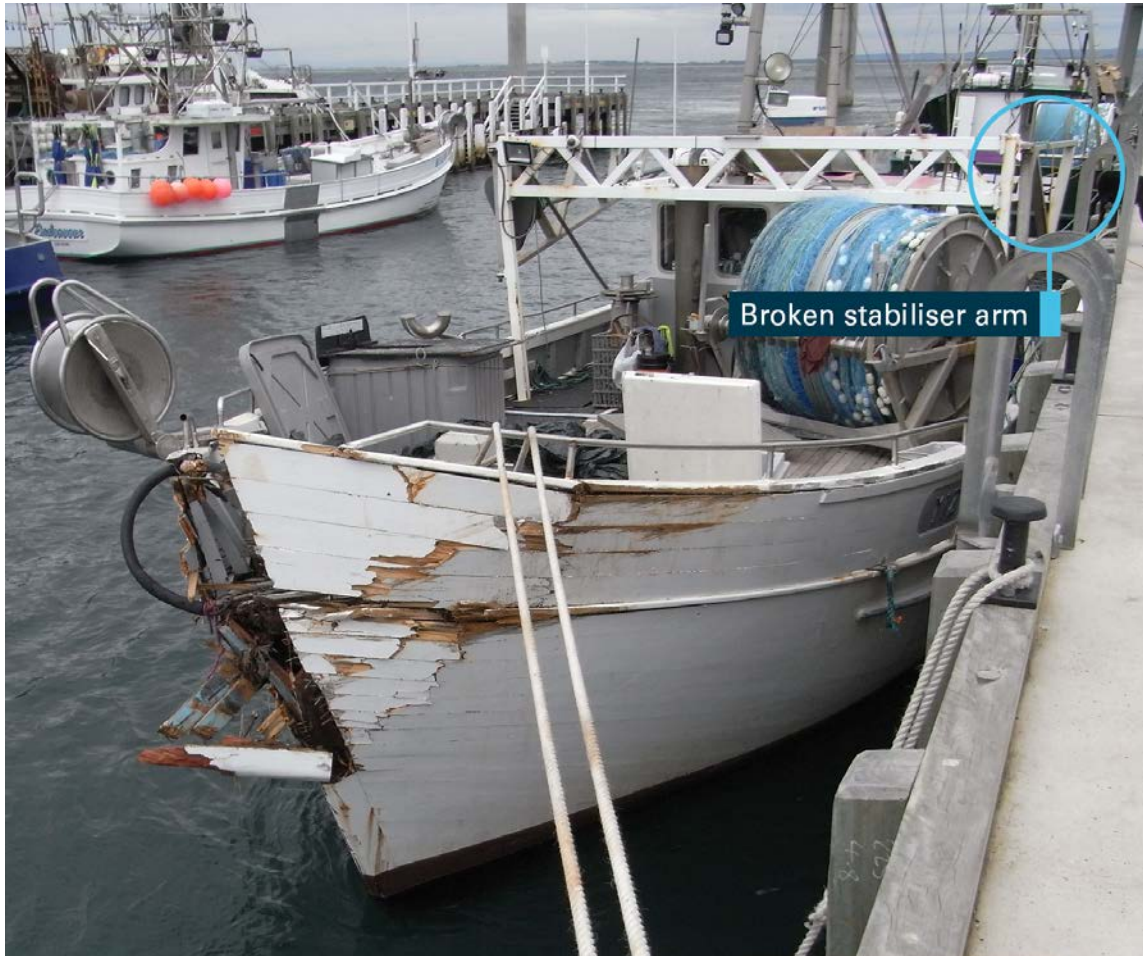
Figure 5: Damage to Mako .
