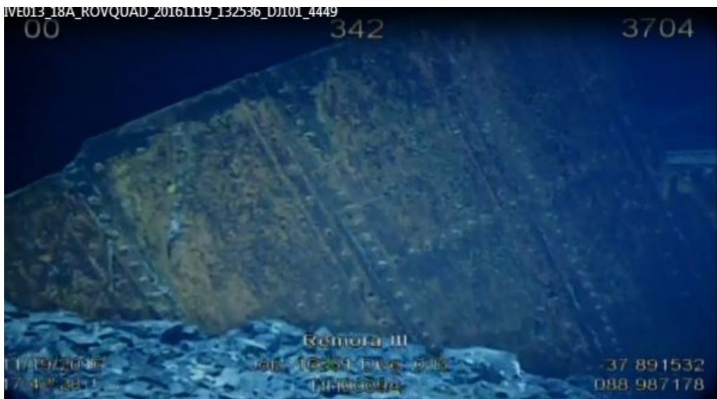
Figure 41 Iron hull plating showing riveted iron frames and hull plating, with remains of coal cargo visible in foreground (ATSB)
