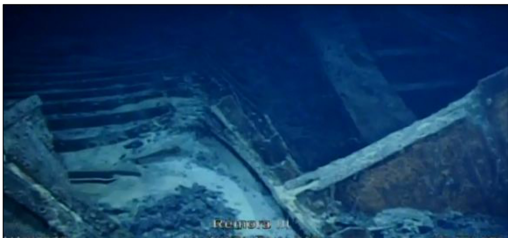
Figure 42 Hull buried in seabed, collapsed outer hull plating (left), collapsed deck (top right) and a bulkhead in the foreground (ATSB)
