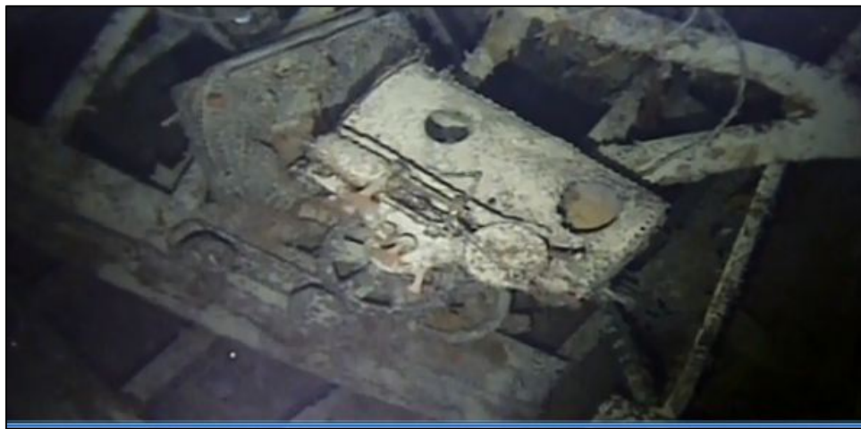
Figure 46 Donkey boiler and machinery (ATSB)
