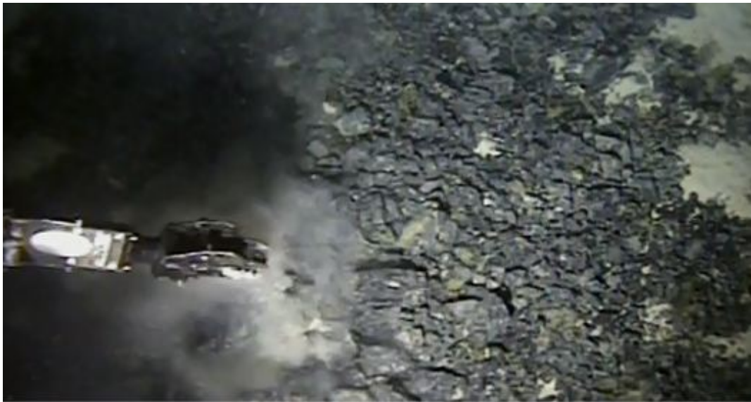
Figure 49 Remora III ROV manipulator arm recovering coal sample (ATSB)
