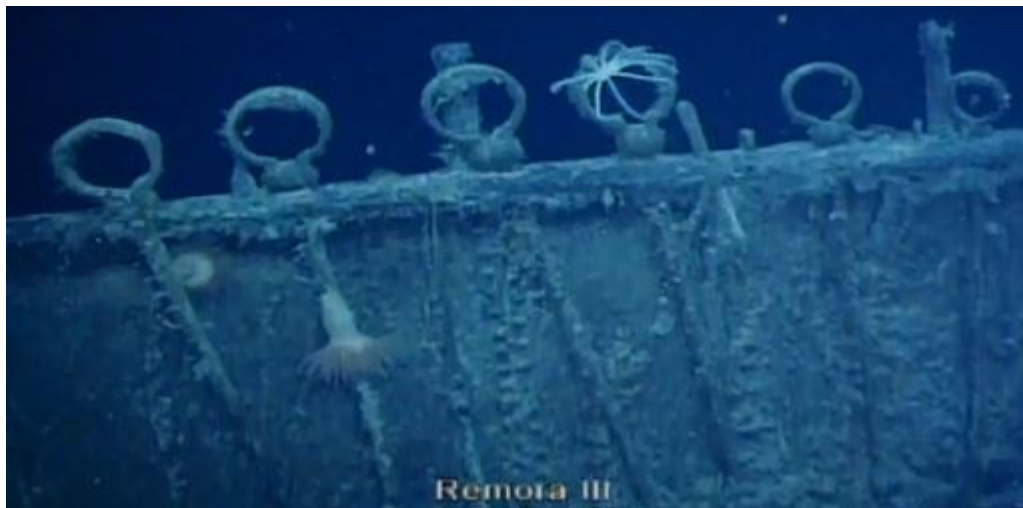
Figure 47 Intact hull with iron rigging chainplates for shrouds, with wooden deadeyes missing. A spider crab and anemone are visible (ATSB)
