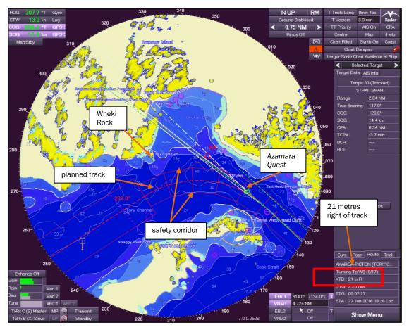
Figure 10 The Azamara Quest was 21 metres off track when the pilot ordered three degrees of port helm
