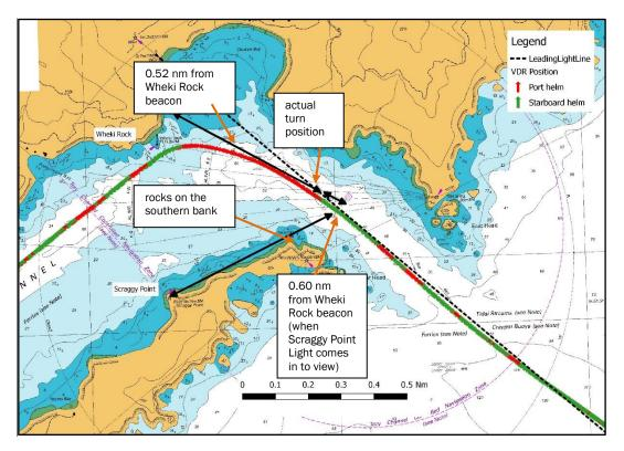
Figure 8 Delay in ordering the start of turn
