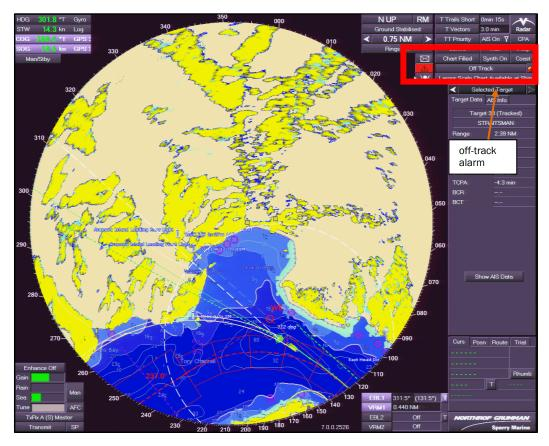
Figure 12 Off-track alarm triggered at about 0919
