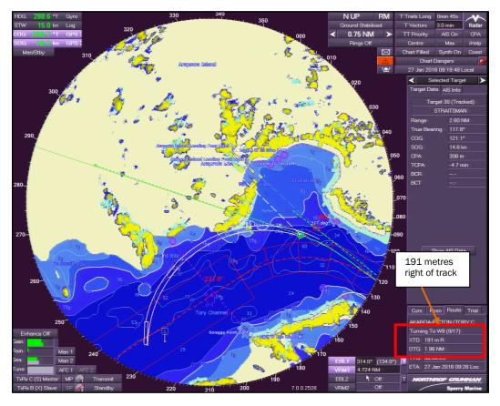
Figure 13 The Azamara Quest was 191 metres off track when the pilot ordered 20 degrees of helm
