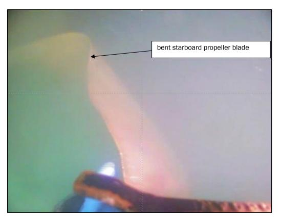
Figure 3 Bent starboard propeller blade
