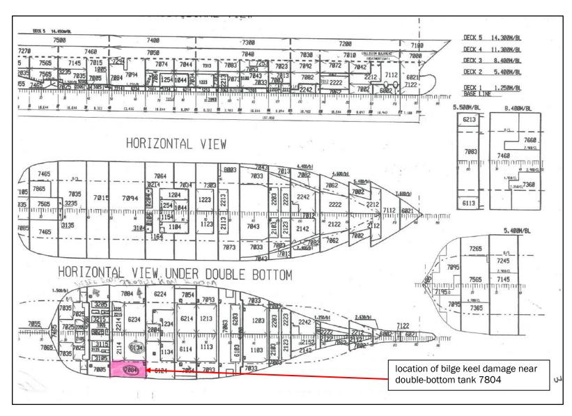
Figure 4 Damage to bilge keel near double-bottom tank 7804
