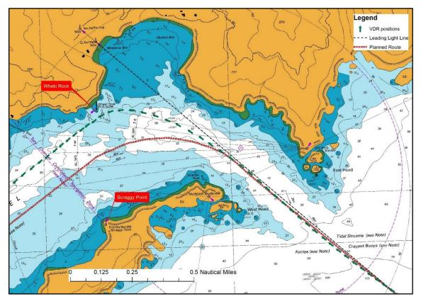
Figure 2 Voyage data recorder positions showing deviation from the planned track
