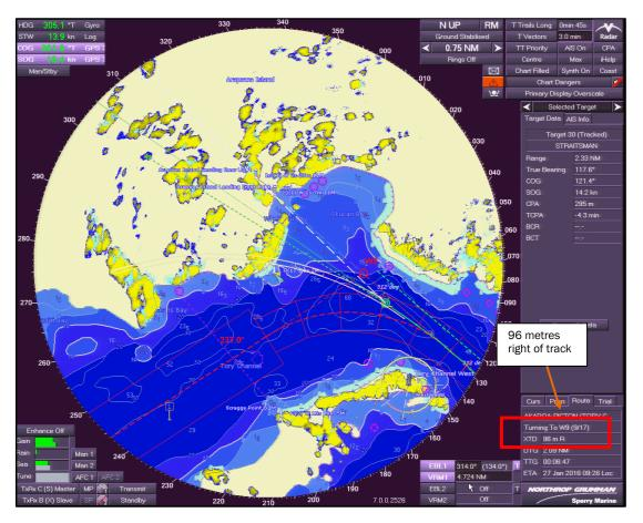
Figure 11 The Azamara Quest was 96 metres off track when the pilot ordered 10 degrees of helm
