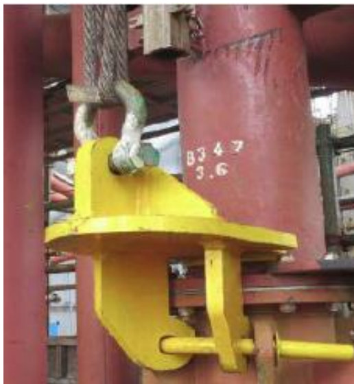
Illustration 11: Lifting yoke to lift riser sections for raw water pumps.
