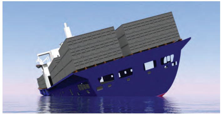
El Faro computer rendering in static surface water showing list to port of 18° with departure trim 5.8 feet by the stern due to flooding of hold 3 estimated at 20% and windheel.
