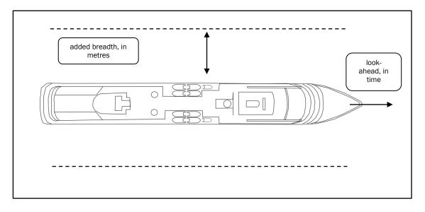
Figure 11 Description of ECDIS time and distance safety parameters
