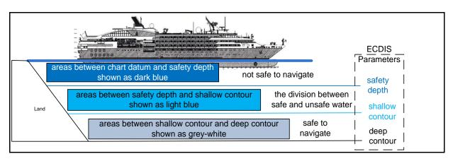
Figure 10 Description of ECDIS depth parameters
