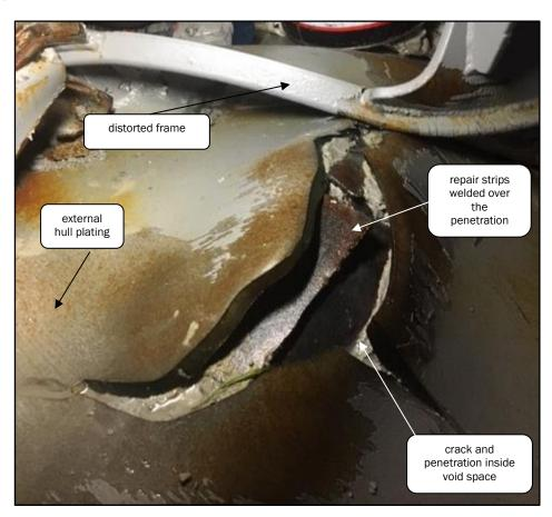
Figure 6 Damage inside the void space
