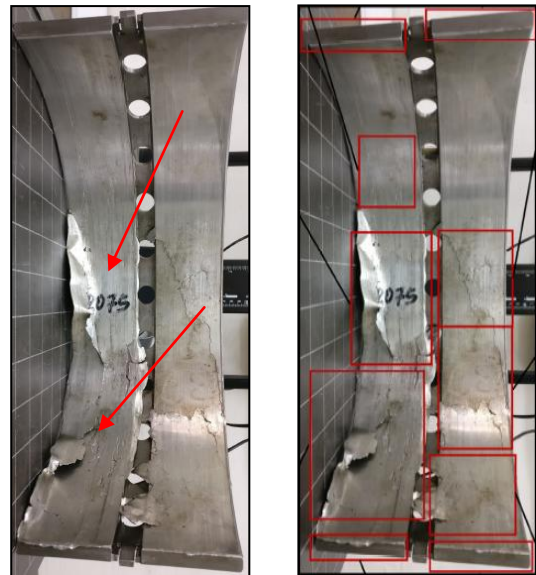
Figures 3a and 3b: Clean separation on the bearing shells
