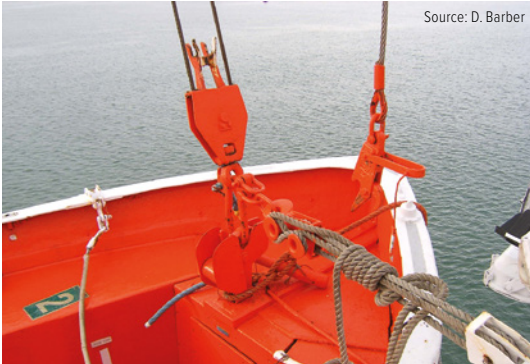
Off-load release. The hook can only be opened if the load is relaxed, as would occur when the boat becomes waterborne.
