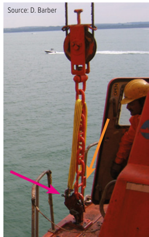
An on-load release hook with FPD attached at hanging-off lug (magenta arrow).
