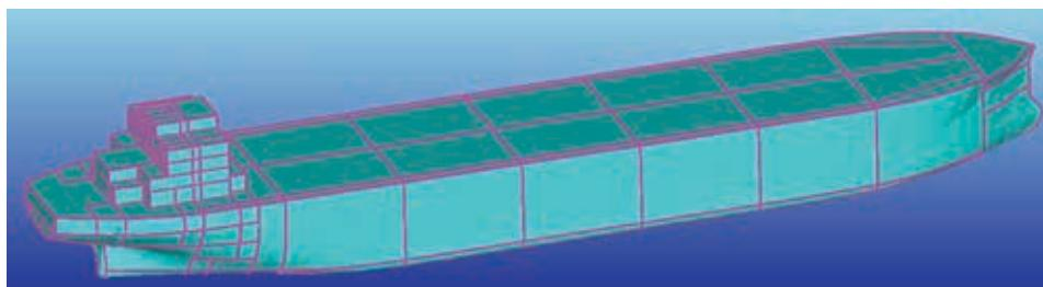
compartment noise level is the combination of the machinery noise and the HVAC noise. Analysis results are evaluated against the relevant noise limit. If the predicted results exceed allowable noise limit, ABS can propose mitigation options for reducing noise levels.
